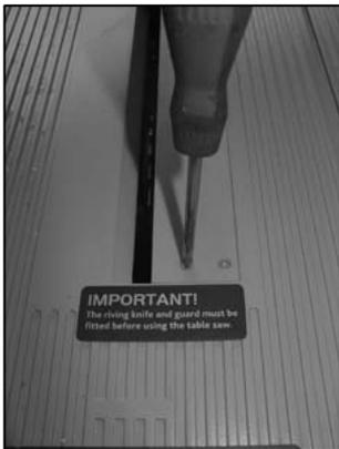
1. Unscrew the screw that fix the protective cap to the riving knife and remove the bench inlay by unscrewing the 8 flat-headed Phillips screws (Fig. 9).
