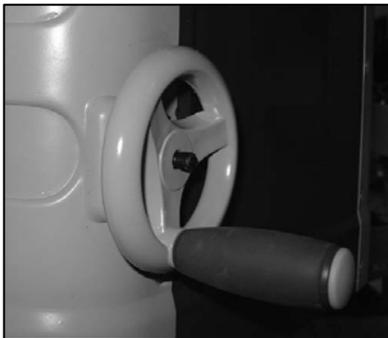
You can use this handwheel to angle the blade (Fig. 21). Turn it clockwise to angle the blade to the left. Turn it anti-clockwise bring back the blade at 90°. Be sure to have loosened the knob located at the level of blade's height adjust knob before angling the blade and be sure to have blocked it when you have chosen the position.
