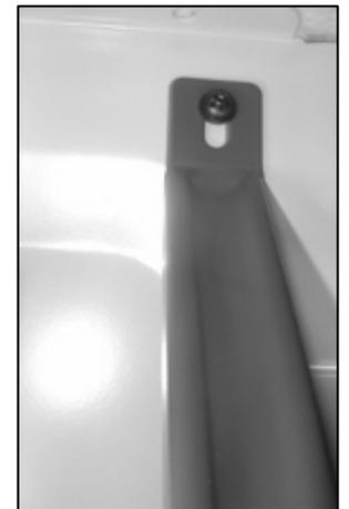
2. Use 2 M5 x 20 mm screws with the washers to fix the supporting parts (L) to the saw's base.
