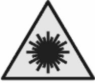
Indicates that this machine is equipped with a laser pointing device (see par. SAFETY INSTRUCTIONS FOR THE POINTING DEVICE).
