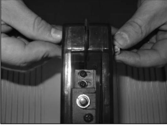
2. Remove blade's protective cap by unscrewing the stop square neck nut. You can also remove the protective cap from the riving knife.
