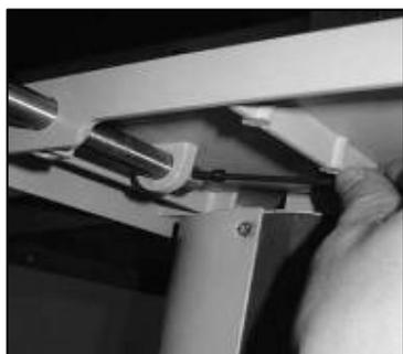
1. Make the bars of the side extension (G) slide on the surface of the table saw.
