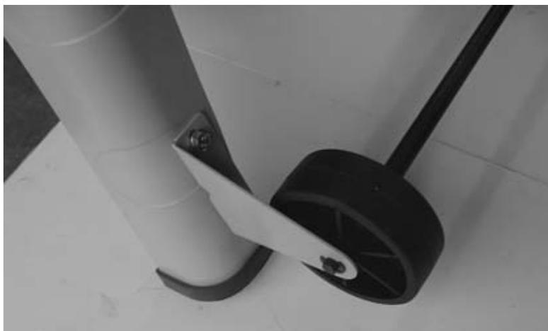
1. Fix the wheel lock supports (O) to the angle posts of the base (H) by using M6x16 mm screws with the washers and the nuts.
