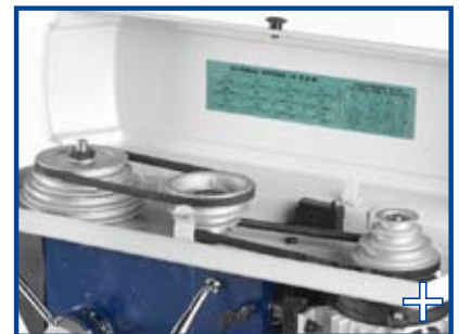
Top cover with safety micro switch
